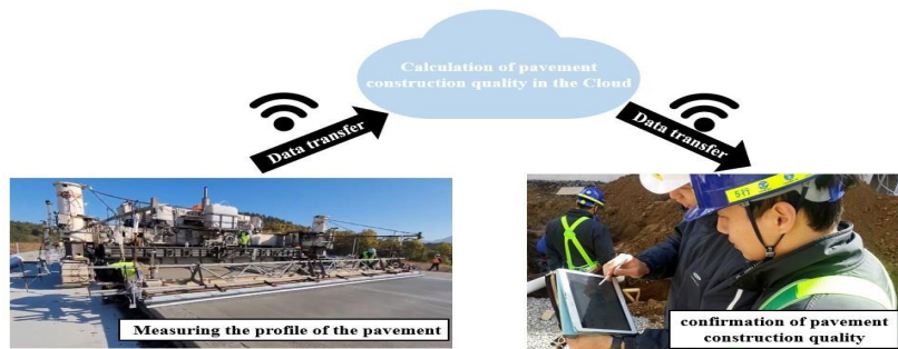
Figure 1-3 Cement Concrete Pavement IRI Measurement System Using IoT
