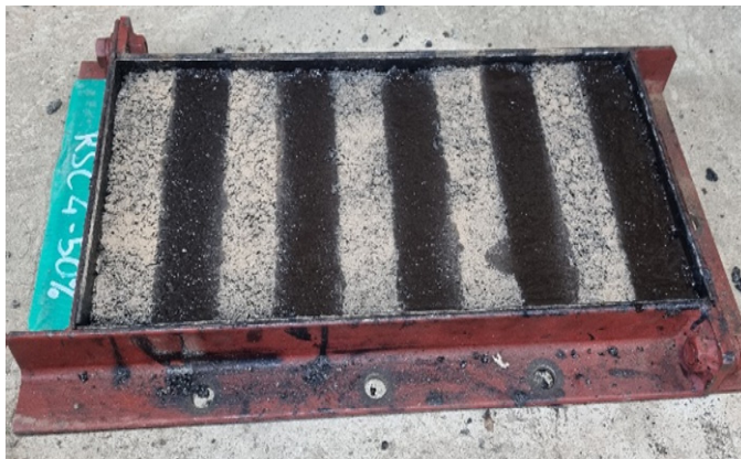
Figure 1. Four-point bending test of tack coat sample
